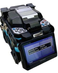
TM-16S Fiber Optic Fusion Splicer is designed as a highly flexible instrument, sturdy structure, easy to use with 4 motor precise micron level control and low loss. TM-16S's 4.3 inch high-resolution color LCD touch screen, anti-reflective with user-friendly intuitive GUI offers large and clear fiber images to users. Fast 8 sec second splicing, 25 second heating features enable TM-16S to be an efficient tool for fiber installation and maintenance.
